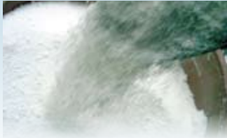
Figure 1: Protected PotCarb, open container, 2 weeks, ambient conditions.
