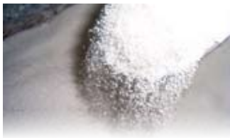
Figure 3: Protected PotCarb, open container, 2 weeks, stressed conditions.
